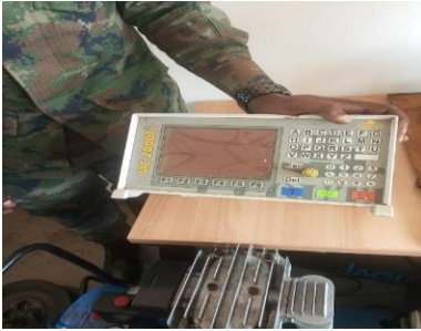
Picture 8: A controller box in Rwanda whose screen and frame are damaged.
