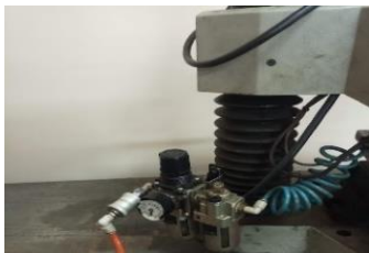
Picture 4: Focus on the pressure system. This was indicated as the most vulnerable part of the equipment.
