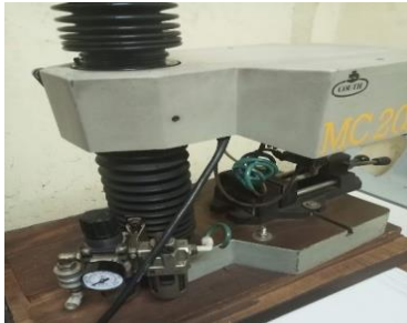
Picture7: The marking machine in Rwanda whose pressure gauge is broken, and the pipe is also damaged.
