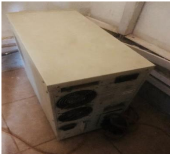
Picture 20 and 21: The above photos show the two pieces of UPS that have failed because of a power surge. The white one was the first and replaced with the black one which has now blown as well.
